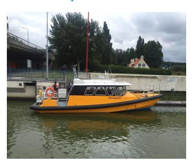
The Windspeed MK3 is an updated version of the Windspeed series featuring an aluminum hull and waterjet propulsion, increasing the reliability over the previous series.
